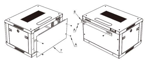
9: Install the Rear panel (7) and the Rear suspension (8), Secure with M5 Screws(A).
