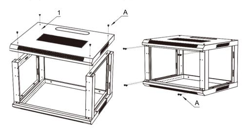
2: Place the Top Panel (#1) onto the Front Frame (#5) and the Back Frame (#6). Secure with M5 Screws(A).
