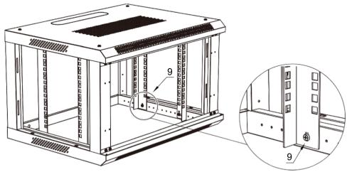
3: Install the 4 Vertical Mounting Rails (#9) into place at the desired depth using M5 Screws(A)for each Vertical Mounting Rails (#9).
