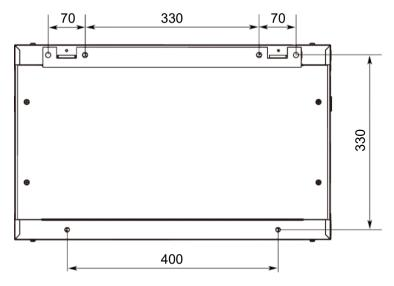
1: Attach the rack to a wall or other suitable mounting surface using M10 Expansion screws(G). The mounting hole distance is shown in Fig, apart to accommodate standard stud placement as reflected in the diagram.
