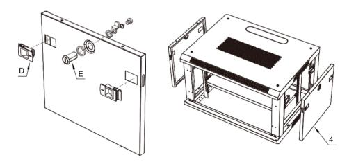
5: Install the Side Panel Latches (D) and the Side Panel Locks (E) on the two Side Panels (#4).
