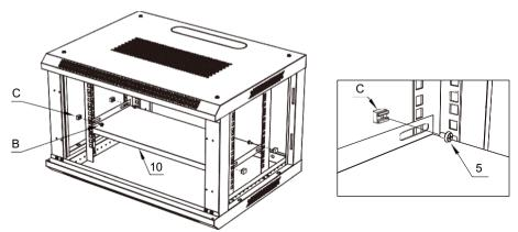
4: Install the Pallet (#10) into place at the desired height ,Secure with M6 Hex Head Screws (B) and M6 Cage Nuts (C).
