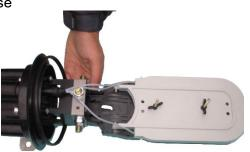
(8) put the cover of the joint box on the base case and tighten it
