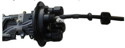
(4) insert the strengthen core into strengthen core retainer, tighten the plastic nut with wrench.
