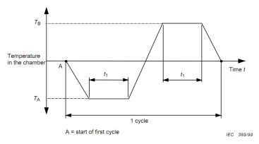
Temperature range:  $T_A$ : - 40 °C;  $T_B$ :60 °C Duration of temperature plateau  $t_1$ : 8h Rate of temperature changing: 1 °C/min
